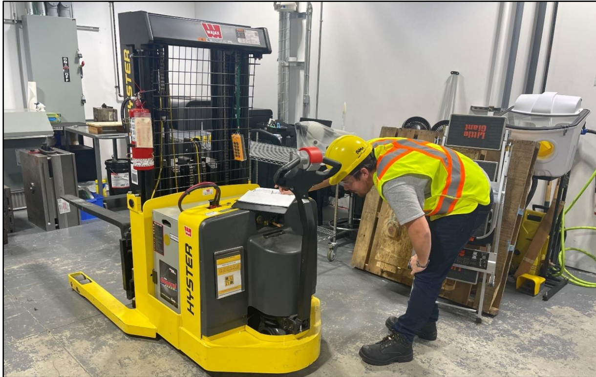
Figure 25: A qualified operator conducts and records pre-job checks of an electric forklift used in support of SRBT's plastics molding processes.
