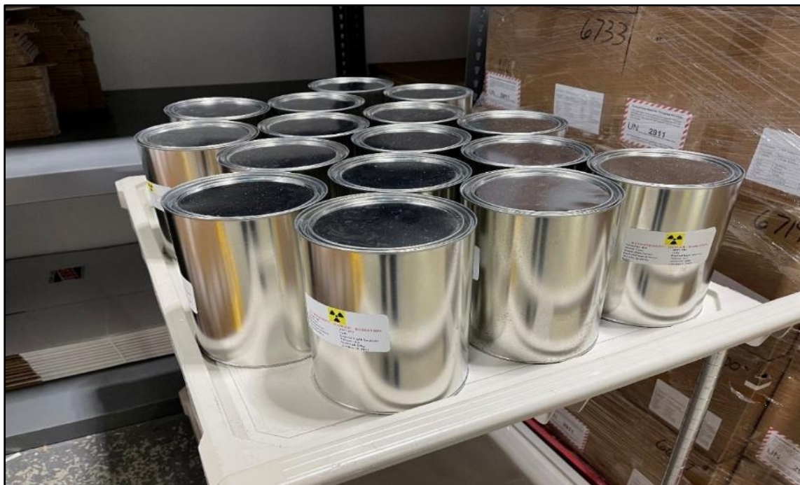
Figure 35: Non-reusable gaseous tritium light sources from expired self-luminous safety signs are placed in Type 'A' shipping containers and sent to a licensed radioactive waste management facility.
