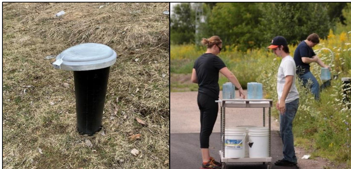
Figure 30: An example of a sampling well at SRBT (left); workers conduct groundwater monitoring at the facility (right). Groundwater monitoring has been continuously performed by SRBT since 2006.
