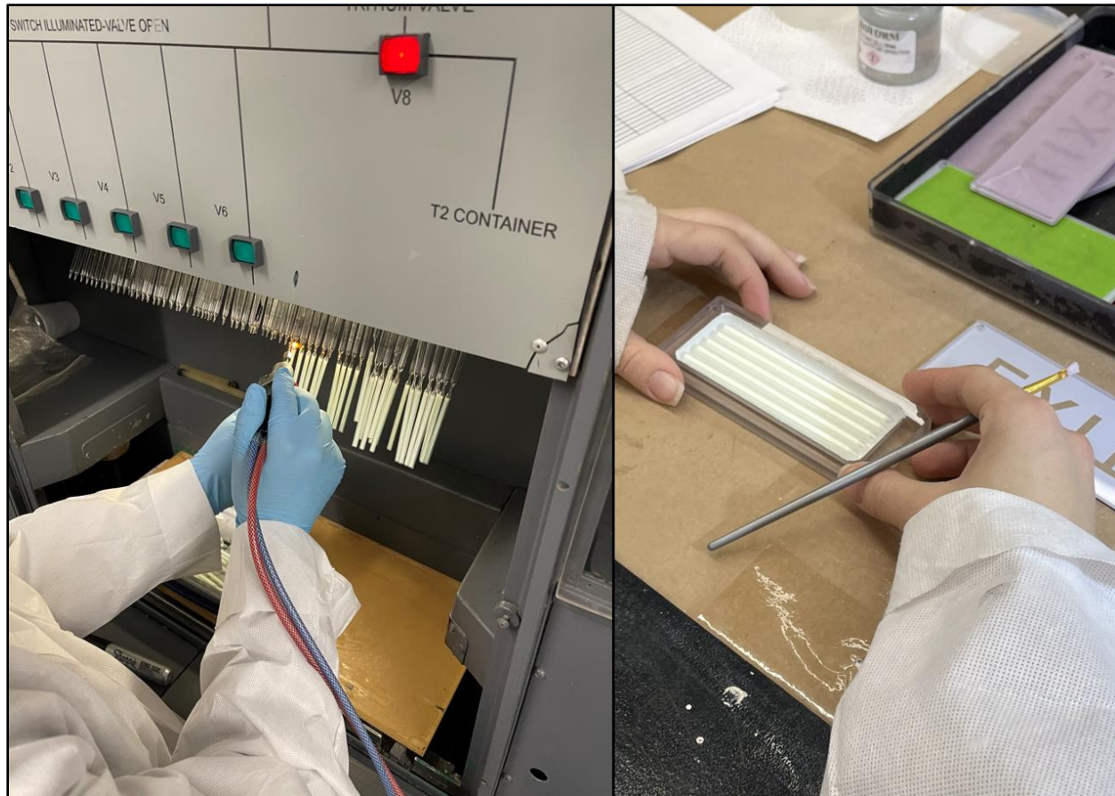
Figure 20: A qualified production technician end-seals gaseous tritium light sources (left); the assembly of a self-luminous aircraft safety sign (right).
