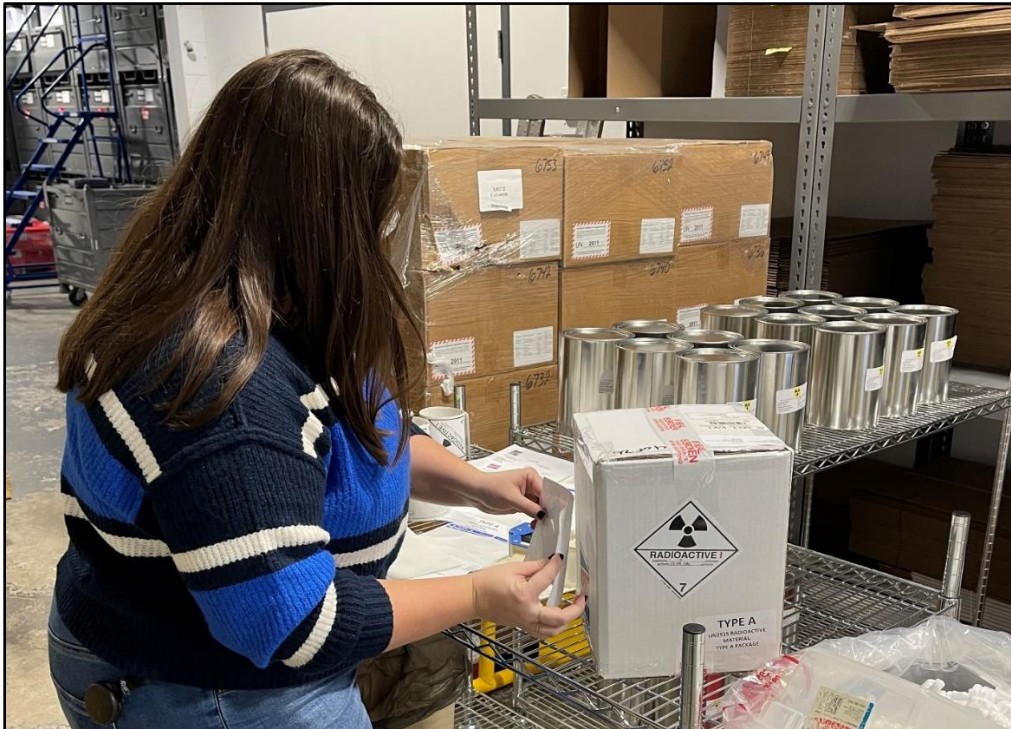
Figure 36: Type 'A' packages of light sources are prepared for shipment, in accordance with the Packaging and Transport of Nuclear Substances Regulations (2015) .
